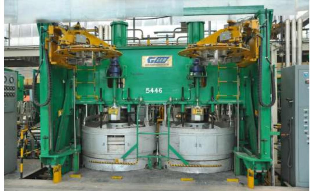
*Platen Type Curing Press in CTP*
